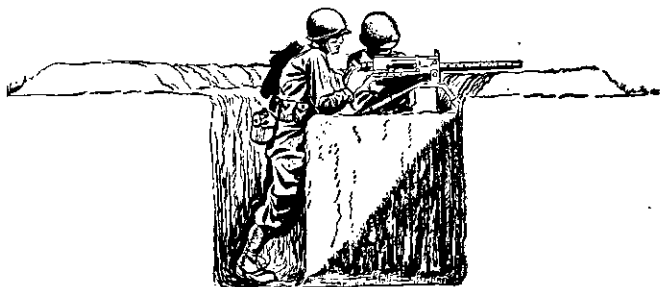
Figure 25. Horseshoe type emplacement for caliber .30 machine gun (light). (Camouflage omitted.)
